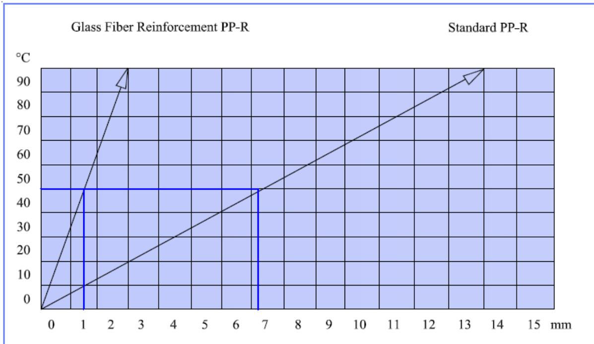
While glass fiber reinforced PPR pipe elongates 1.75mm in 1 meter at temperature difference of at 50°C, on the other hand standard PPR pipe elongates 7.5mm in 1 meter in the same temperate difference
